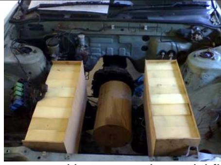
The motor and battery mockups trial-fitting.
