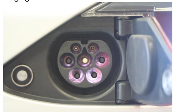
Pic: Tesla modified Type 2 socket (note notch at top to prevent use of Tesla Superchargers with normal Type 2 sockets). Source: Wikipedia
